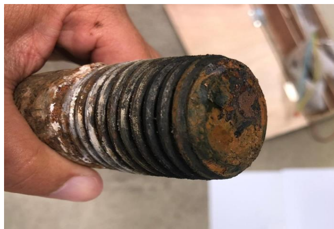
Figure 3-8 A corroded threaded rebar under examination
